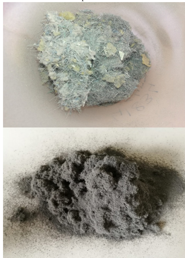
Figure 1. 1-a (left): the whole waste sample as crushed <4 mm in the cutting mill for the leaching test, according to standard EN 12457-2; 1-b (right): the whole waste sample as ground <1 mm in the centrifugal mill.
