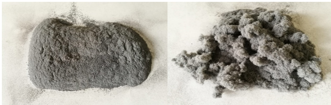
Figure 1. 2-a (left): the waste sample as ground <1 mm in the centrifugal mill, fraction passing through a 0,5 mm sieve and predominantly powdery and non-fibrous; 2-b (right): the waste sample as ground <1 mm in the centrifugal mill, oversize fraction through a 0,5 mm sieve and predominantly fibrous.
