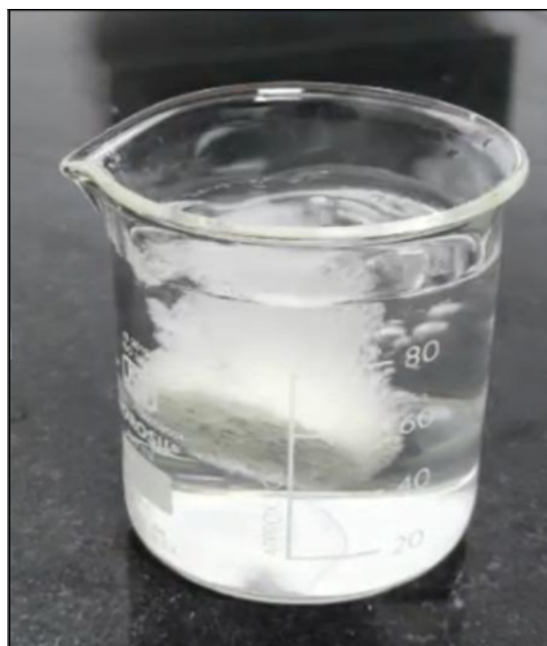
Figure 4. Evaluation of the disintegration/dissolution time of the effervescent tablet in water.
