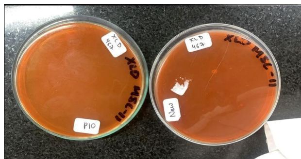
Figure 9. Microbial limit test on Xylose Lysine Deoxycholate agar (XLD) showing absence of Salmonella spp.
