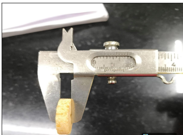
Figure 3. Measurement of tablet thickness using a vernier caliper to check dimensional uniformity.
