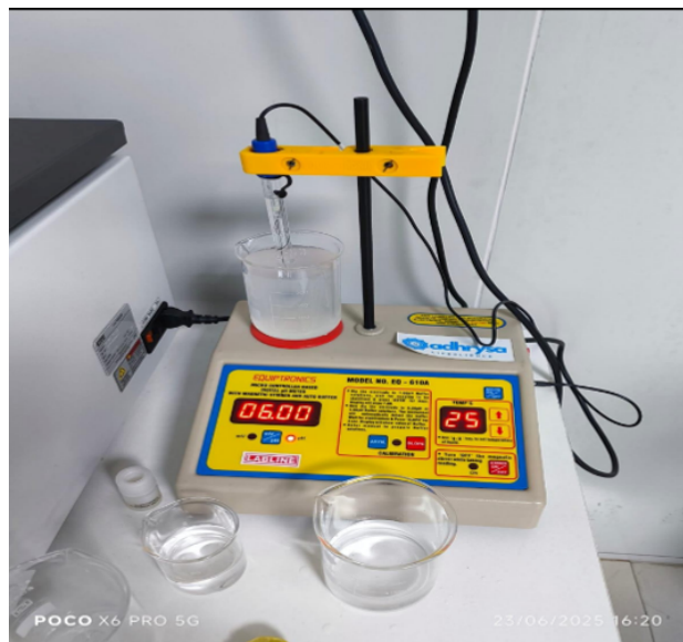
Figure 2. Measurement and determination of the dissolved effervescent tablet solution pH using a digital pH meter (pH = 6.00).
