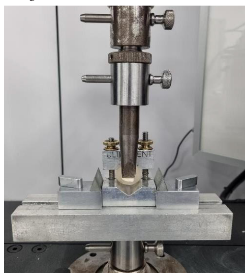
Figure 4. Instron universal testing machine. The pin is applied on the palatal surface of the veneer, 1mm from the incisal edge and with a 90° angle with the axis of the tooth.
