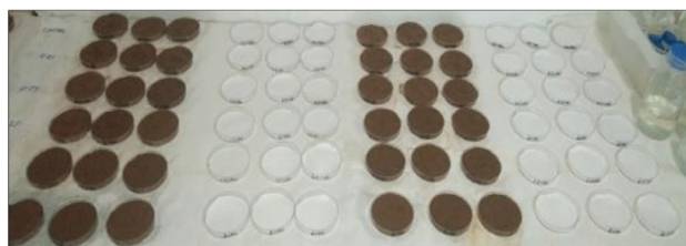
Figure 1. Experimental set-up with soil (brown Petri plates) and blotting paper (white Petri plates) bases.
